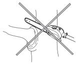
Use the stop at the base of the cutting head to provide support during cutting. This will help prevent the cutting attachment from "jumping" on the branch.
