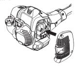
Some mufflers are equipped with a special spark arrestor mesh. If your machine has this type of muffler, you should clean the mesh at least once a week. This is best done with a wire brush.
